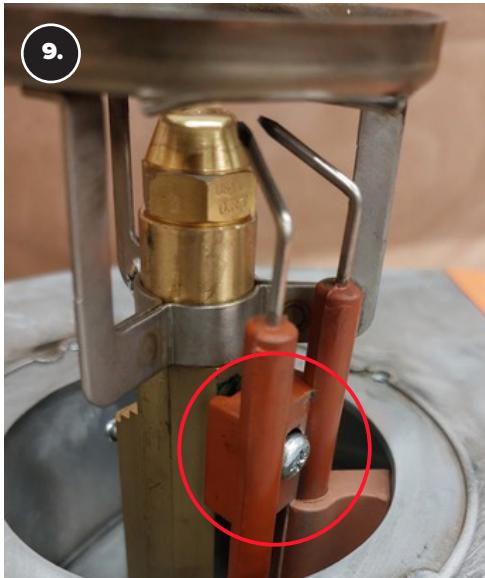
First loosen the igniter screw and loosen the igniter out of the nozzle frame.
