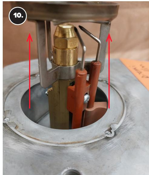
Then remove the air flow diffuser carefully by lifting it up to reveal the nozzle.
